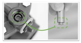
When replacing the solenoid, the plunger needs to be replaced as well. Turn the manual override to 'auto' and detach the plunger sideways (click). Then replace the plunger by clicking it back in sideways.
